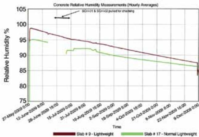
**Fig. 9:** RH results for normalweight and lightweight concrete slabs tested in Study 2, Controlled Environment
