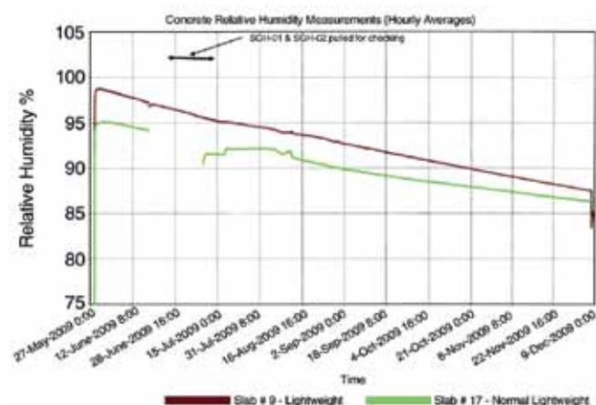
**Fig. 9:** RH results for normalweight and lightweight concrete slabs tested in Study 2, Controlled Environment
