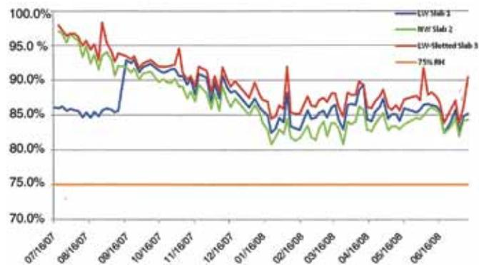
Fig. 5: MVER history for Study 1, Nonconditioned Environment; 1 lb/1000 ft<sup>2</sup>/24 h = 56.5 μg/(s · m<sup>2</sup>)
