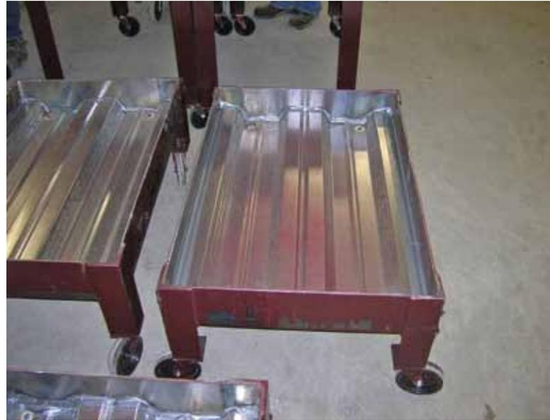
Fig. 7: Test slab formwork used in Study 2
